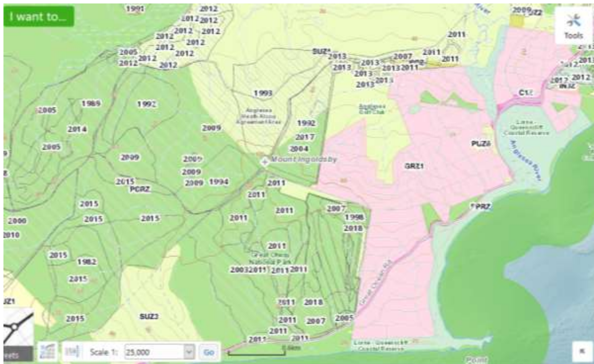
Figure 4 This map shows good evidence of deep and regular control burning around the danger perimeters of Anglesea. Control burning reduces maximum flame height on site which reduces ember generation capability. Low flame stops by itself at fuel free barriers, eg, tracks wider than flame height. Bushfire progress depends on ember throw, which has also been disrupted by regular burning. Regular burning provides habitat renewal for several species and prevents severe fires on site and consequent wide scale burnout, deaths and multi-layer habitat destruction.
