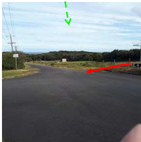
Figure A1n (left) Looking north along the western firebreak. Red arrow indicates direction of NW to SW wind driven running flame through the mown grass, where maximum flame height will be 1m if it cures. Running flame will self-extinguish at road edge, ie, stop without suppression.
