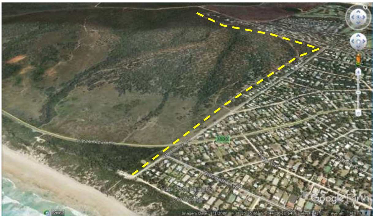
Figure 2 Oblique view to the NW across the SW corner of Anglesea towards the heathy forest mass. This yellow dash line indicates where the running bushfires are stopped from NW, W and SW by the passive protection measures of control burns and wide mown firebreak and wide boundary road.
