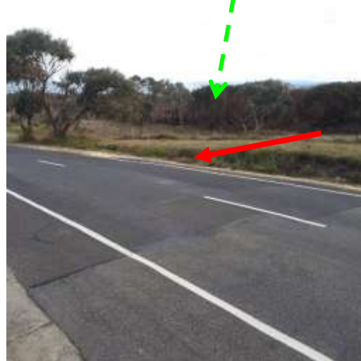
Figure A2s (left) and A2sw (right) Looking south and SW along the western firebreak. Red arrow indicates direction of NW to SW wind driven running flame through the mown grass, where maximum height will be 1m. Running flame will self-extinguish at road edge, ie, stop without suppression.
